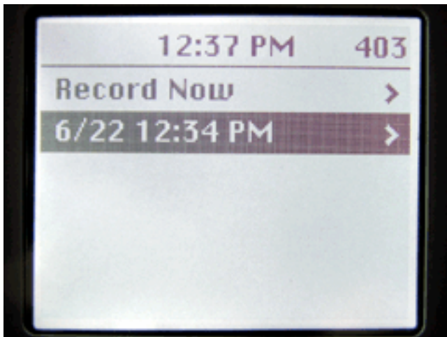
Each recording appears chronologically in the Extras>Voice Memos menu. Selecting a recording offers the choice to play it or delete it.
