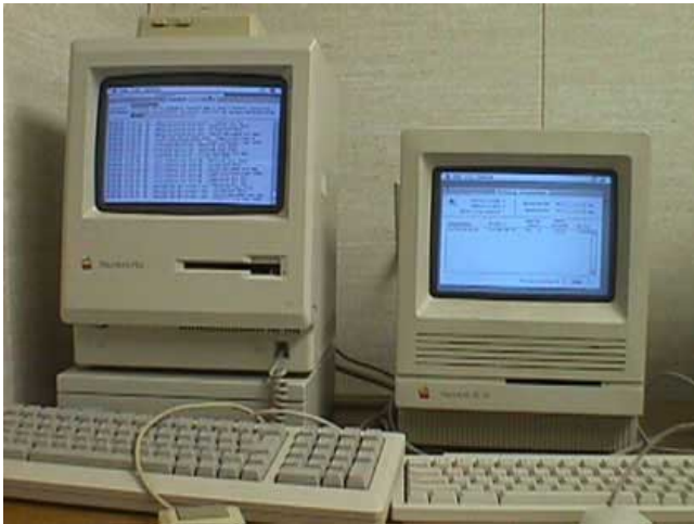
Bob’s Mac Plus with an SE/30 next to it running Apple IP Gateway.
