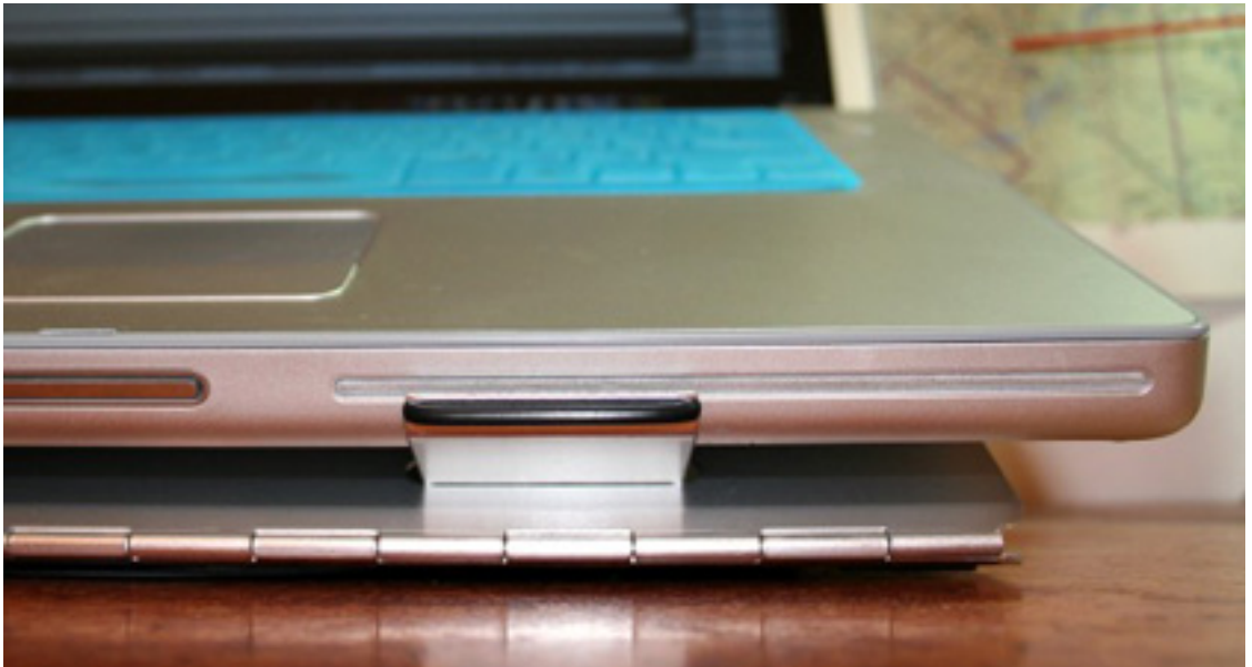
Blocked Optical Drive
