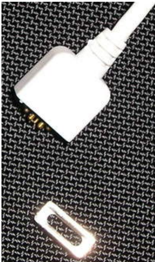
Battery Geek MagSafe Knock Off, Fallen Apart
