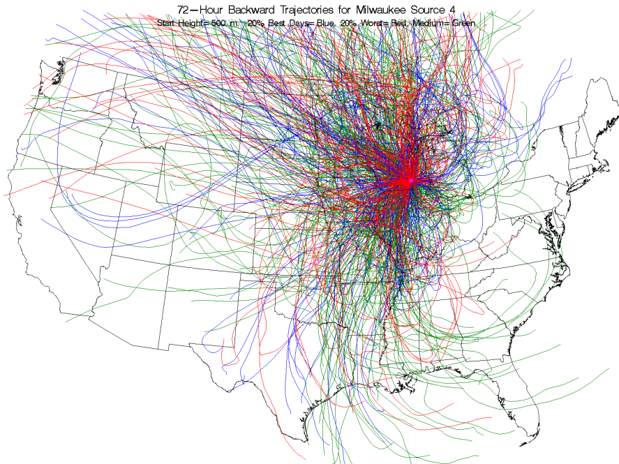
Figure I-23 Back Trajectories Color Coded by Source Strength Category for Milwaukee, Wisconsin, Source 4 - Chlorine Sources.
