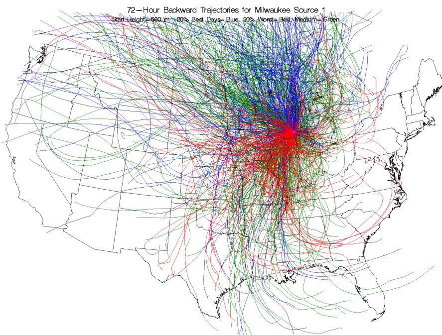
Figure I-5 Back Trajectories Color Coded by Source Strength Category for Milwaukee, Wisconsin, Source 1 - Coal Combustion (Ni).
