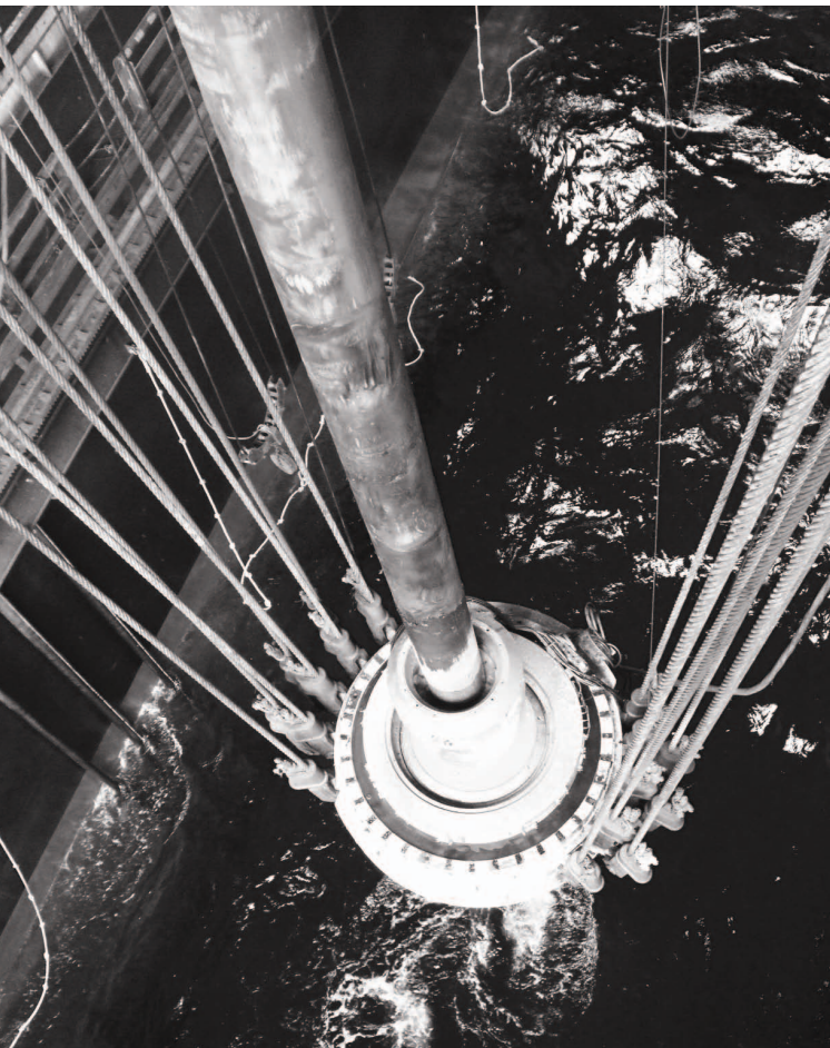
Oil rig riser and slip joint for offshore drilling.
