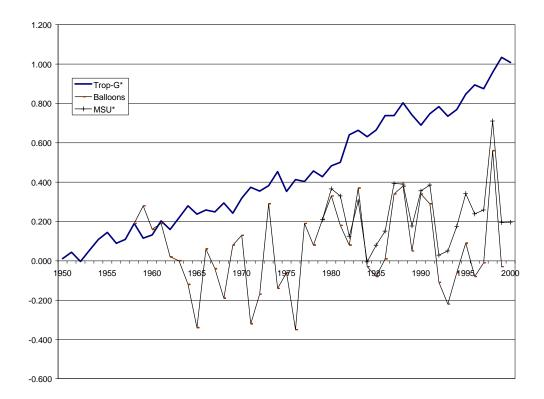
The Trop-G line was generated by a leading climate model, the Goddard Institute for Space Science coupled Atmosphere-Ocean General Circulation Model, forced with  $CO_2$  and sulphate emissions since 1950. The Balloons line is from Angell (2000) and the MSU line is from Spencer and Christy (1990).
